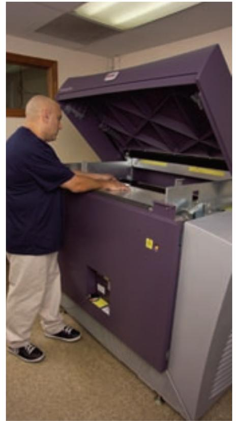
Carmen Demaio positions a plate for imaging on the **Kodak Thermoflex** Narrow platesetter.
